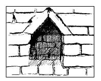
Bee boles were built mostly in walls of stone, but where stone was not the common building material (e.g. Kent), they were made in brick walls. The wall often bounded a garden or orchard. The bee boles usually faced south to south-east so that the bees would be warmed by the morning sun. The base of the bee boles was often two to three feet from the ground, thus at a convenient height for working, although skeps of bees were rarely handled except when the honeycombs were harvested.
