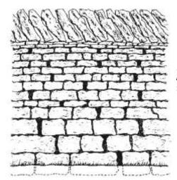
Front elevation showing weep holes in a Yorkshire-style retaining wall
