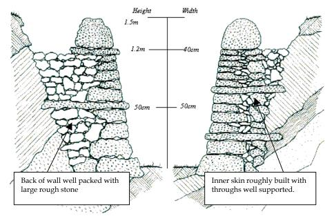
Sections through a Scottish-style retaining dyke and a Yorkshire-style (right) retaining wall.
